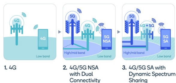
Fig4: 4G/5G Non Stand Alone & Stand Alone with DSS
