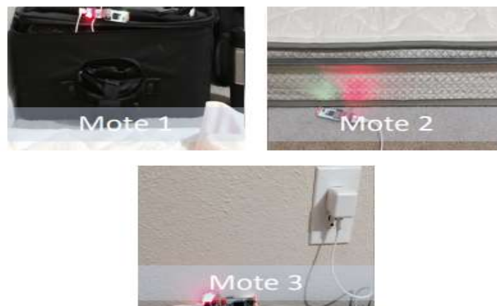
Figure3. Mote 1 (Motion), Mote 2 (Pressure) & Mote 3 (Bend) in Passive Monitoring Unit.
