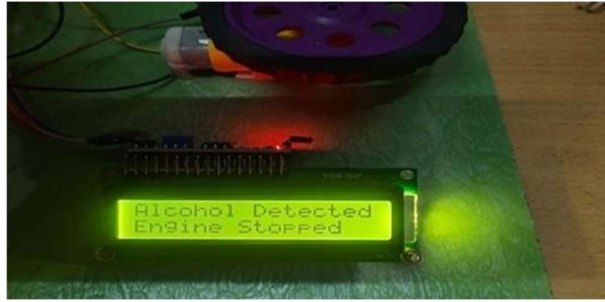
Figure 7 Vehicle Halted Due to Alcohol Detection
