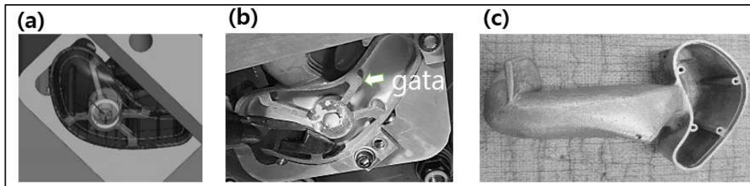
Figure 2: (a) 3D modeling of the tool path for removing casting gates, (b) Mounted on jig to remove casting gate (c) A cyclic stick product after casting gate removal processing.
