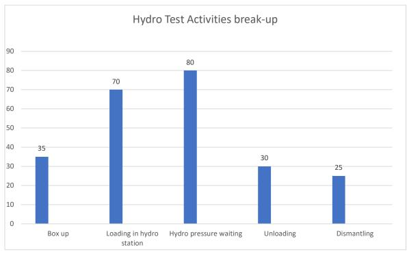
The Hydro-test process for pumps involves several critical activities that must be completed accurately to ensure that the test is successful. The first step is to box up the casing and seal chamber tightly, ensuring that no water can escape during the test. This is done by placing flanges in the suction and drainage sections of the casing, a process that takes approximately 35 minutes to complete.
