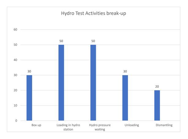
The graph provided depicts the results of the changes we made to the hydro-testing process. The data clearly shows that the use of a pneumatic torque gun significantly reduced the time required for various activities such as boxing up, loading, unloading and dismantling the casing and seal chamber from the hydro-station. Specifically, the time for each of these activities was reduced by 5 minutes each. This means that the overall time saved by using a pneumatic torque gun was 20 minutes.
