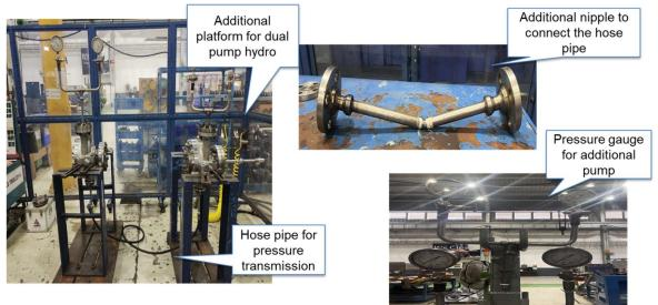
The results we got from the above setup is given below, the hydro-test activities break up after improvement is given below.
