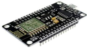
The microcontroller known as the ESP8266 was created by Espressif Systems. The ESP8266 is a self-contained Wi-Fi networking system that can execute standalone programs and serves as a bridge between Wi-Fi and current micro controllers. This module includes a built-in USBconnector as well as a wide range of pin-outs. Similar to Arduino, you can easily flash the NodeMCU devkit by connecting it to your laptop using a micro-USB wire. Additionally, it is right away breadboard friendly.
