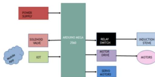
Figure 4- Block diagram of a new automatic cooking machine
