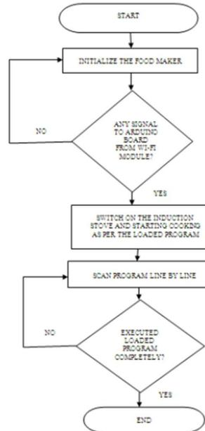
Figure 6- Flow chart for Wi-Fi controlled automatic food maker
