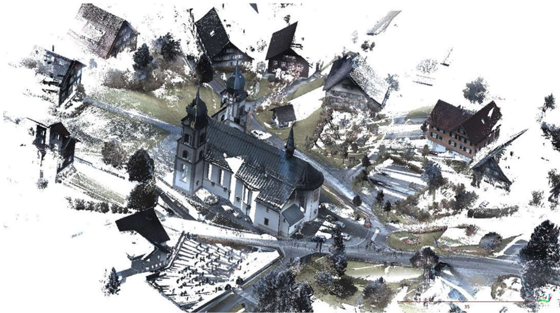
Figure 3: Example of cloud in Semantic3D dataset (3 clouds registered). Occlusions, density depends on the distance to the LiDAR.
