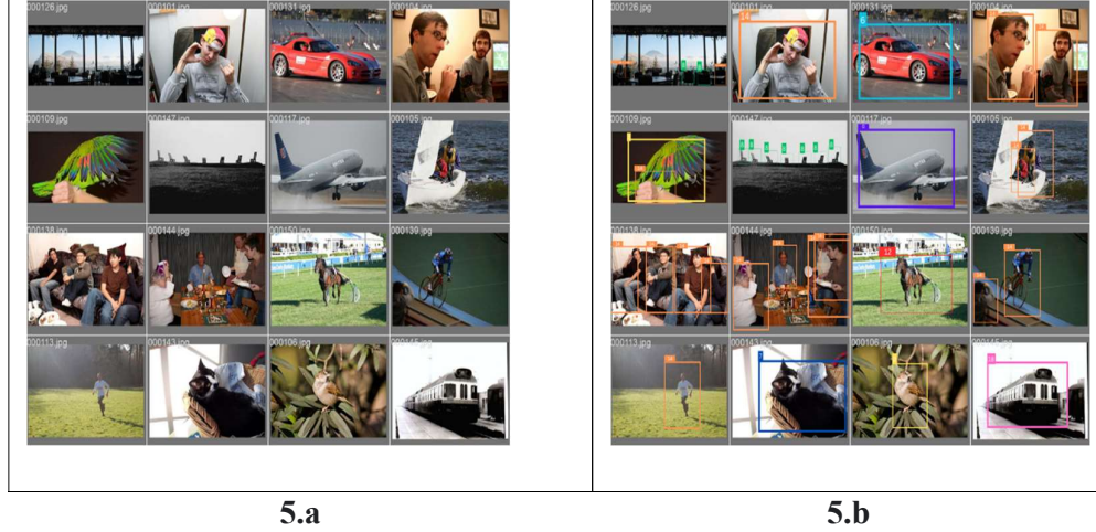
Fig. 5.a) Sample Input of image with multiple objects 5.b) Output of the proposed Custom Deep Convolutional Neural Network CDNN
