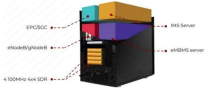
Amarisoft Callbox is a solution provided by Amarisoft, a company specializing in 4G and 5G network technologies. Callbox is a test tool designed to simulate a mobile network, allowing users to test various aspects of their network equipment and applications.
