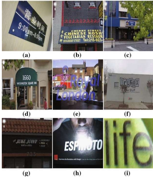
Figure 1: Examples of scene text detection problems. Different orientations; different languages; different colours; different sizes; e complex background; f occlusion; g blur; h noise; i non-uniform illumination (Xiyan Liu et al 2019)
