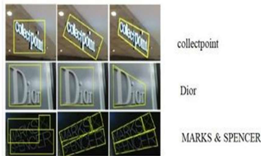
Fig 3.2: Recognizing text from image
