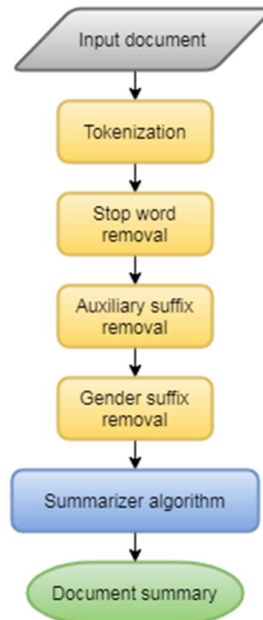
Fig. 1: Block diagram of the extractive text summarization architecture
