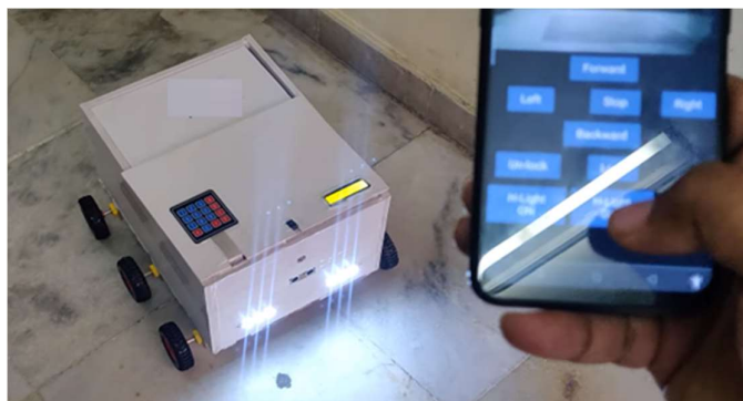
Fig: controlling head lights from WEB Application
