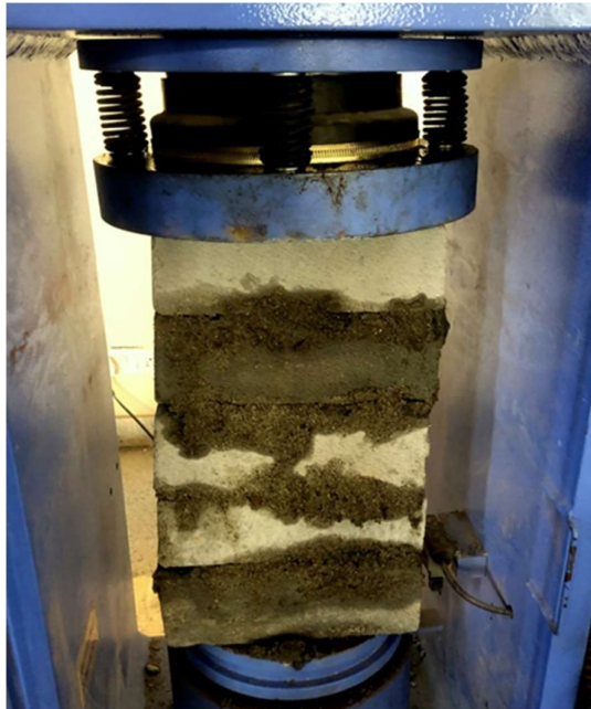
Figure 11. Configuration in the loading frame
