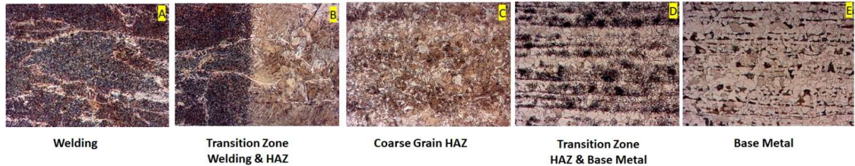
Figure 7. Microstructure study from welding to plate zone
