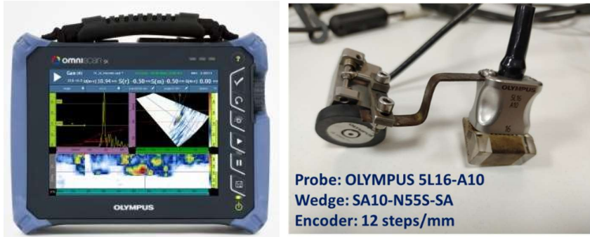
Figure 8: details of Phase array ultrasonic testing machine and probe specification
