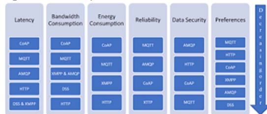
Fig. 2.2.1: Communication Protocols in Industrial Environments
