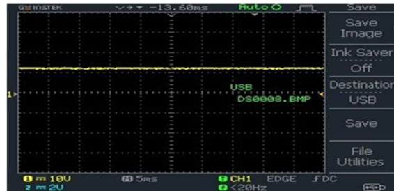
Fig.13. (b) flyback converter output voltage V_{dc2}
