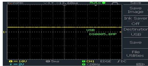
Fig.13. (a) flyback converter output voltage V_{dc1}
