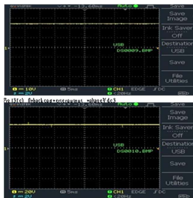
Fig.13(c) flyback converter output voltage V_{dc3} The eight unipolar switches in the 31-level ASCHBMLI arrangement at the 31-level output voltage level with a total harmonic distortion of 2.15 percent without employing any filters. The harmonic norm of IEEE 519 is met in term of percent total harmonic distortion (THD).
