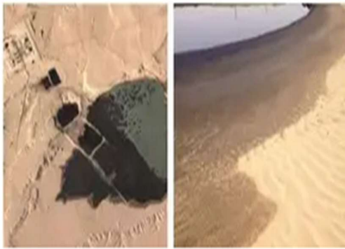
Fig1- Oil contaminated sand caused by produced water
