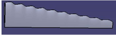
Fig 3(b) Wavy Tapered wing ( \frac{1}{2} th of the distance of semi wing)
