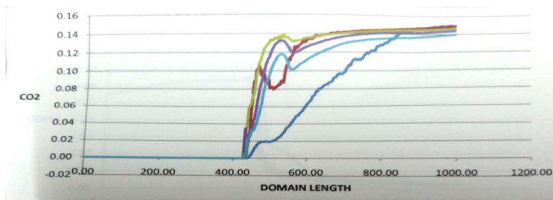
Figure 13: Graphical representation of CO 2 mass fraction of combustion chamber with stepped cavity flame holder
