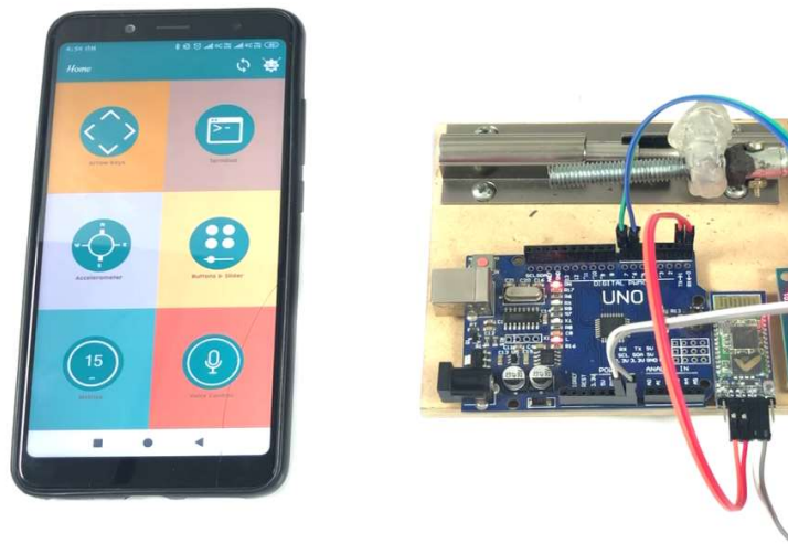
Figure (7)-Door locking system using Bluetooth technology
