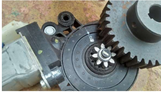
Fig. 3. Spur Gear attached with BLDC Motor
