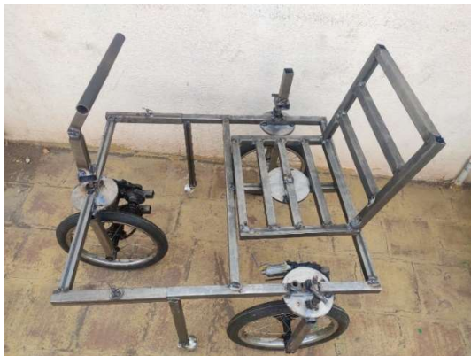
Fig. 1. Mild Steel Square Body Frame Work
