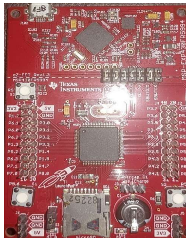
Photograph1 overview of MSP-EXP430FR5994 Launch Pad Development Kit. The photograph 1 shows overview of MSP-EXP430FR5994 Launch Pad Development Kit.
