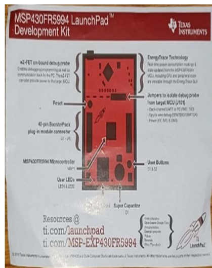
Photograph1 overview of MSP-EXP430FR5994 Launch Pad Development Kit. The photograph 1 shows overview of MSP-EXP430FR5994 Launch Pad Development Kit.
