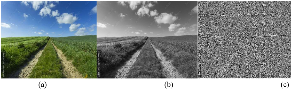
Fig.5 (a) Input agricultural lane image (b) Gray scale conversion image (c) edge detected image
