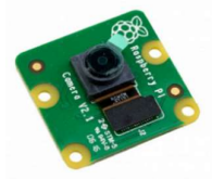
Figure 3.2 : Raspberry Pi Camera with 5Mega Pixel
