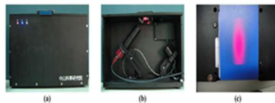
Fig. 2.1: - The prototype of the proposed laser speckle is capturing device (a) appearance, (b) interior, and (c) bird's eye view with blue plastic card.
